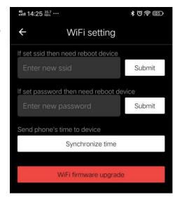
**Note:** If the device is reset to the factory settings, the name and password of the Wi-Fi will also be restored to the default settings.
