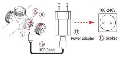
**Note:** It only supports charging the built-in battery pack, not the replaceable 18650 battery.
