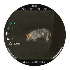
Reticle Style ( - = ): Rotate the Controller (7) to select the reticle style, and press the Controller (7) to switch among 7 styles.
