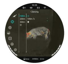
Rotate the Controller (7) to move the reticle position, until the reticle center aims at the position
