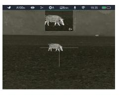
For example, when the magnification of the main image is 3×, 6×, 9×, 12×, the corresponding magnification of the PIP image is 6×, 12×, 18×, 24×.
